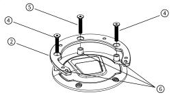
3. Place part 1 on top of part 2 (note to align the holes), put in the screws, and tighten the screws in turn. (Torque: 1.5N·m)
