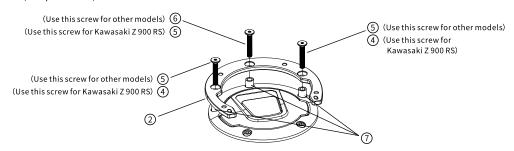
3. Place part 1 on top of part 2 (note to align the holes), put in the screws, and tighten the screws in turn. (Torque: 1.5N·m)
