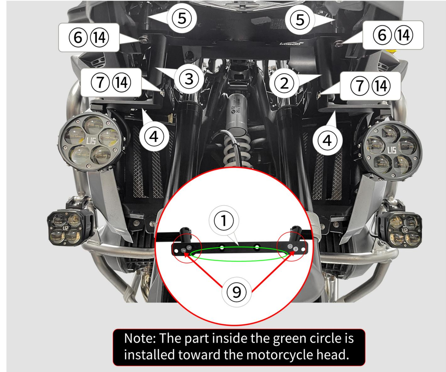
Note: The part inside the green circle is installed toward the motorcycle head.
